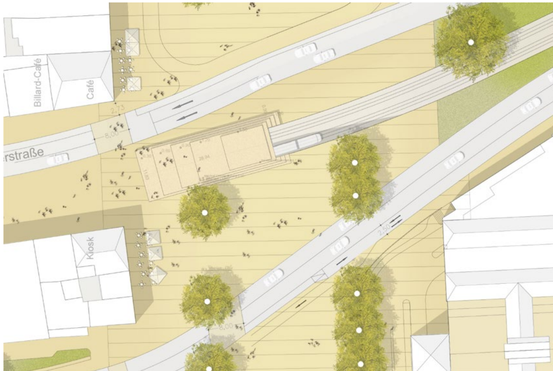
Light rail underground, short tunnel variant, Section 1: Heumarkt, Variant 1: Tunnel mouth as a pedestal
