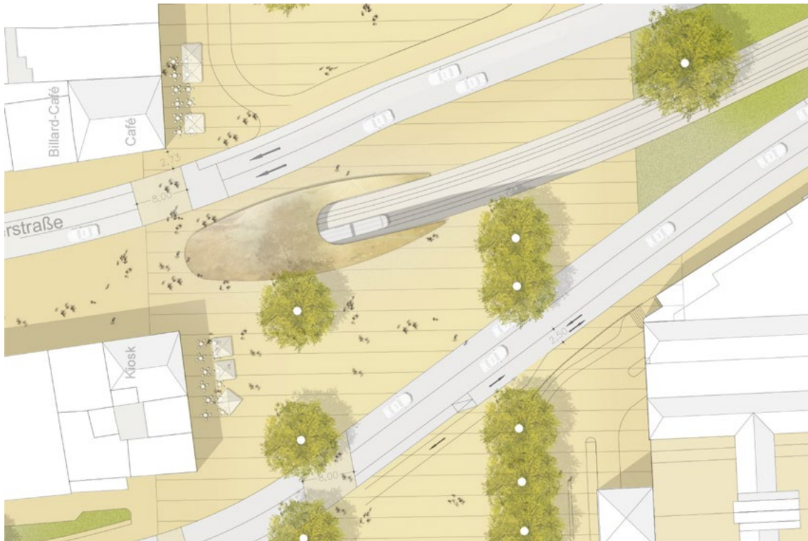
Light rail underground, short tunnel variant, section 1: Heumarkt, variant 2: tunnel mouth as a sculpture
